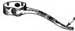
Flyback Lever Spring Assembly No. 17
